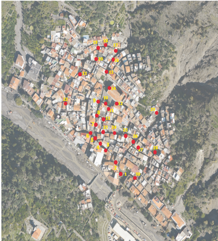
Figure 6. Orthophoto of Giampilieri urban area with positions where data of maximum flow depths and final sediment deposits are available from site surveys.
