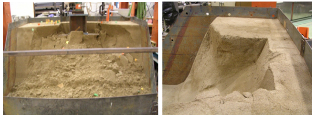
(c) Final failure state after failure mass (d) global failure surface after failure mass is removed
