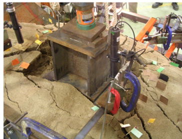
(e) Penetration of base plate into the soil
