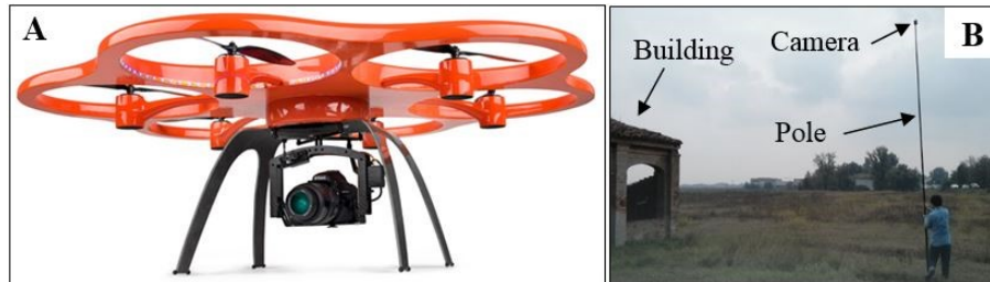
Figure 2. The two platforms used to collect data. (A) Aibot X6 V1 UAV, (B) camera attached to a pole.
