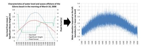
**Figure 5.** Evolution of the sea conditions near Gâvres during Johanna storm (sea level from MARS simulations, significant wave height and peak period from SWAN simulations) on the left, and reconstitution of a corresponding time series of water level with the DIWASP toolbox on the right.
