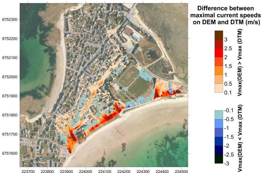
**Figure 12.** Difference between the maximum current speeds obtained inland during the SURF-WB simulations, with and without an explicit representation of the buildings ( $V_{\max \text{ DEM}} - V_{\max \text{ DTM}}$ ).
