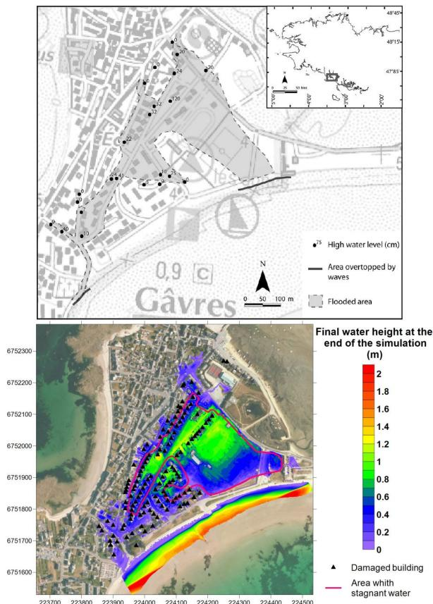
**Figure 9.** Above: measurements of maximum water heights (Cariolet, 2010); below: final water height at the end of the SURF-WB simulation and reported flooded buildings and stagnation area according to the municipality (from the Gâvres municipality and Le Cornec and Peeters, 2008).
