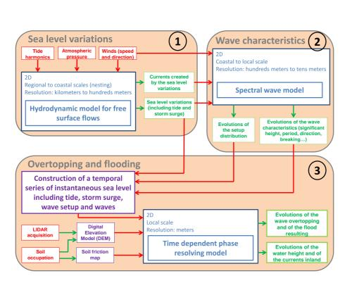
Figure 1. Modelling method proposed to simulate wave overtopping and associated flooding.
