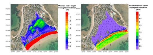
**Figure 11.** Maximum water heights (left) and currents (right) obtained inland during the SURF-WB simulation on the DTM (without explicit representation of the buildings).
