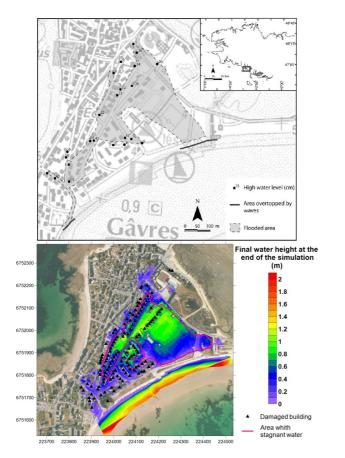
**Figure 9.** Above: measurements of maximum water heights (Cariolet, 2010); below: final water height at the end of the SURF-WB simulation and reported flooded buildings and stagnation area according to the municipality (from the Gâvres municipality and Le Cornec and Peeters, 2008).
