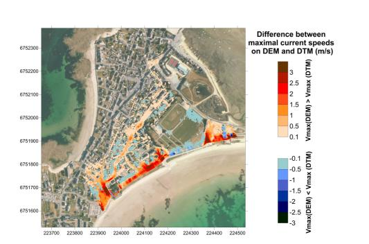
**Figure 12.** Difference between the maximum current speeds obtained inland during the SURF-WB simulations, with and without an explicit representation of the buildings ( $V_{\text{max DEM}} - V_{\text{max DTM}}$ ).
