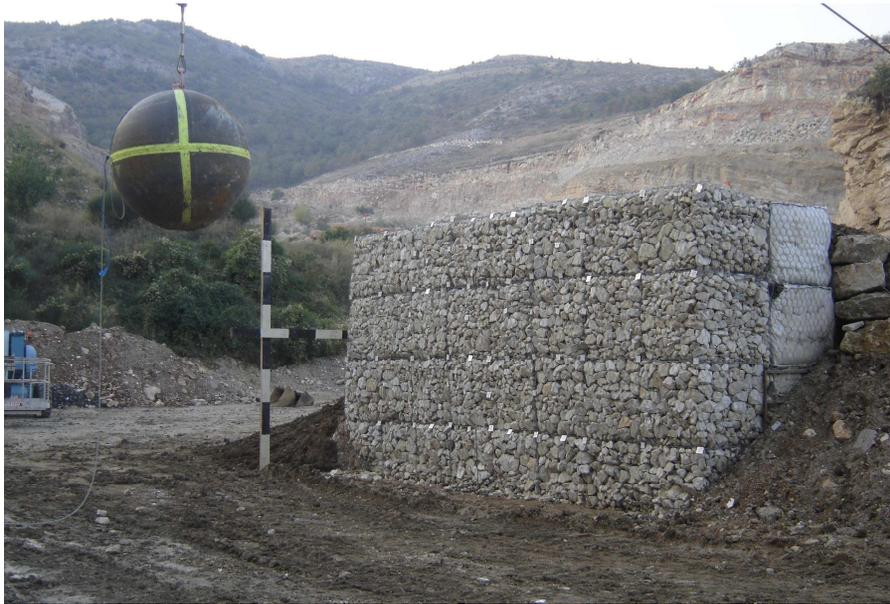
**Fig. 1.** View of the tested embankment, showing the sandwich wall leaned against the levee and the hanging projectile.
