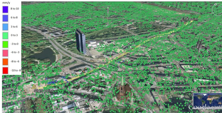
Figure 5. 3-D view of velocity map, displayed on Google Earth. The yellow line indicates the approximate location of tunnelling.
