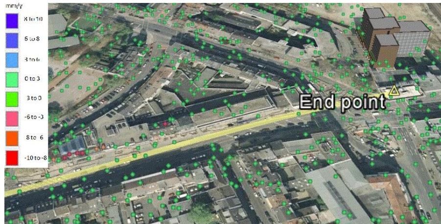
Figure 8. PS points close to the end point of the tunnelling excavation, displayed on Google Earth. The yellow line indicates the approximate location of the tunnelling line.
