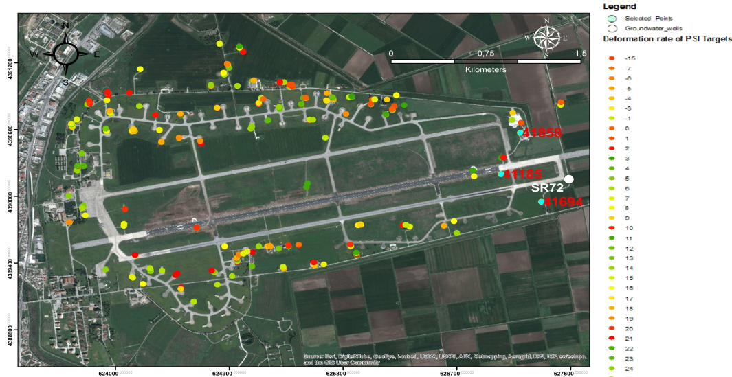
Figure 5. Average LOS velocity image along the runway and areas of Larissa National Airport for the period 1995 to 2006. The image has been saturated at \pm 0.1 \text{ m year}^{-1} for visualization purposes. The numbered persistent scatterers with cyan color have been extracted and analyzed to evaluate time series of ground deformation. Background is base map world imagery white point is the borehole R72.
