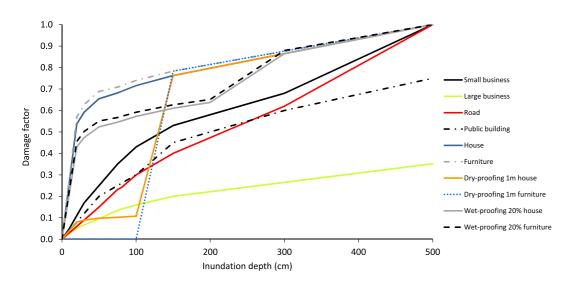
Fig. 3. Stage-damage curves as used in this study, including examples of dry and wet-proofing.
