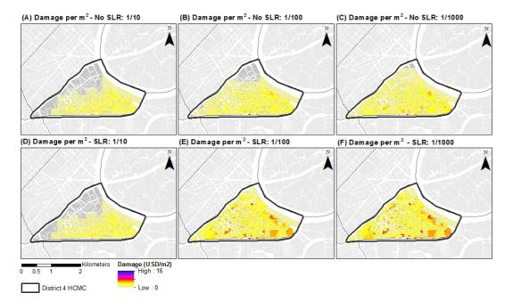
**Fig. 6.** Damage occurring for floods with different return periods, the top figures **(A–C)** are baseline sea level, and the bottom figures **(D–F)** result from using the sea-level rise scenario.
