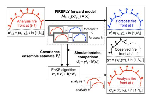
**Figure 2.** Flowchart of the EnKF algorithm during the [t - 1, t] assimilation cycle for a SE approach.
