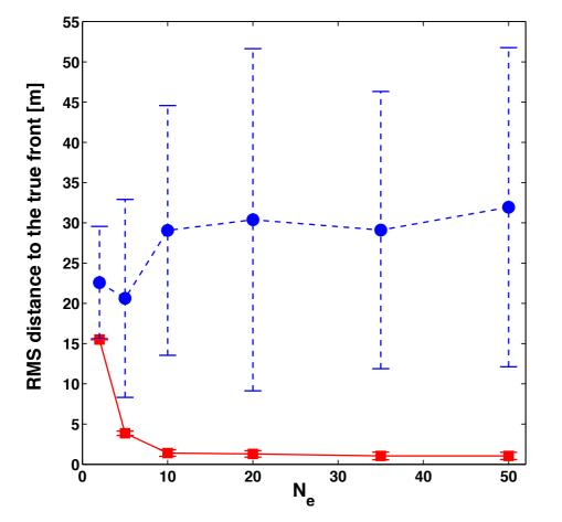
**Figure 8.** Average distance between the true and forecast fire front positions (blue circles) and between the true and analysis fire front positions (red squares) at time 150 s as a function of the number of members  $N_{\rm e}$  in the ensemble; OSSE anisotropic case. Error bars indicate the associated STD.
