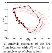
**Figure 5.** Spatially-varying OSSE test with uncertain ROS model parameters and with uncertain ignition location ( $x_{ign}$ ,  $y_{ign}$ ); one assimilation cycle; all figures correspond to time t = 150 s. (a) Comparison between true (black solid line) and forecast (blue dashed lines) fire front positions. (b, c) Comparison between true (black solid line) and analysis (red dashed lines) fire front positions. Black cross symbols are the  $N_{fr}^{o}$  observed front markers.
