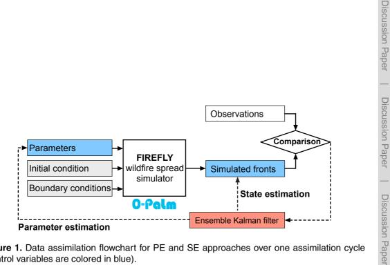
Figure 1. Data assimilation flowchart for PE and SE approaches over one assimilation cycle (control variables are colored in blue).
