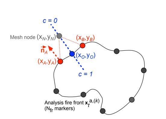
**Figure 9.** Schematic of the reconstruction algorithm for the FIREFLY initial condition. In this example, the mesh node  $(x_N, y_N)$  is outside the burnt area, the inner product  $(\overrightarrow{ON} \cdot \overrightarrow{n_A})$  is positive.
