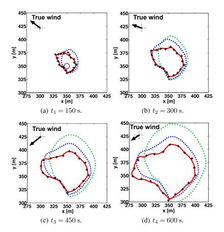
**Figure 11.** OSSE anisotropic case over multiple assimilation cycles (from 0 to 600 s): comparison between the free run (green dashed-dotted line), mean forecast estimate (blue dashed line), observations (black crosses) and mean analysis estimate (red solid line) at 150 s time intervals, at times (a)  $t_1 = 150$  s (the gray circle corresponds to the true initial location); (b)  $t_2 = 300$  s; (c)  $t_3 = 450$  s; and (d)  $t_4 = 600$  s.
