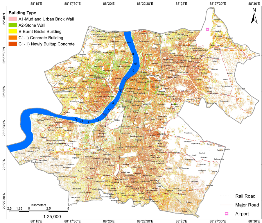
Fig. 6. Building typology distribution map of Kolkata derived using LISS IV and LANDSAT TM imagery.
