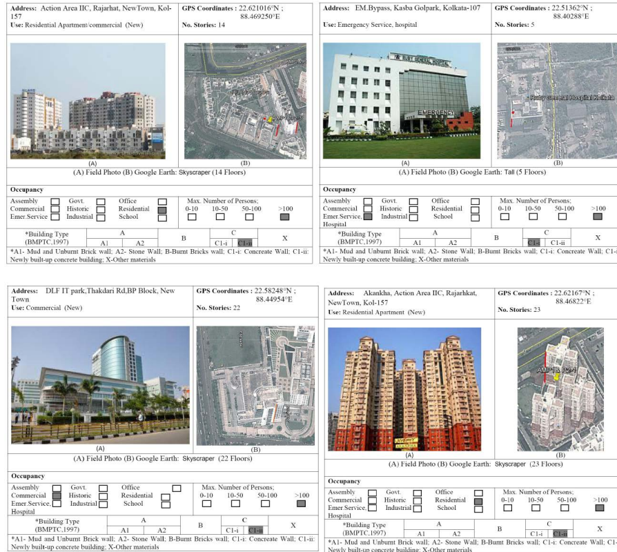
Fig. 3. Rapid Visual Screening (RVS) survey (at about 1200 sites) for field and Google Earth comparisons of existing building height in urban Kolkata for potential seismic vulnerability assessment.
