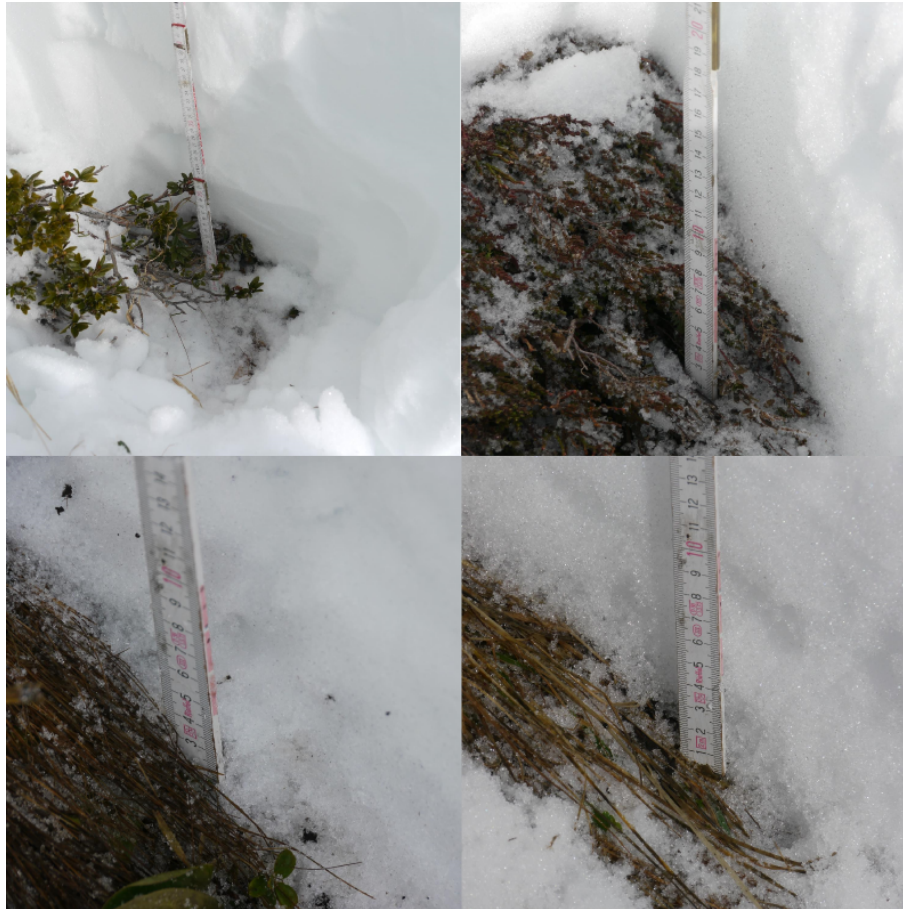
Fig. 4. Vegetation below the snow cover. Vegetation heights h_v are smaller in winter than in autumn: less than one centimeter for long grass, 3 cm for short grass, 4 cm for low dwarf shrubs and 10–20 cm for strong lignified shrubs.
