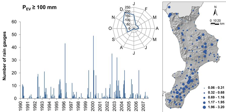
**Fig. 5.** Rainfall events characterized by  $P_{EV} \geq 100$  mm: timeline of the number of rain gauges that exceed the threshold value. The numerousness of events for each month is shown in the inset. The location and the ratio between numerousness of rainstorms and number of observation months for each rain gauge is shown in the map on the right.
