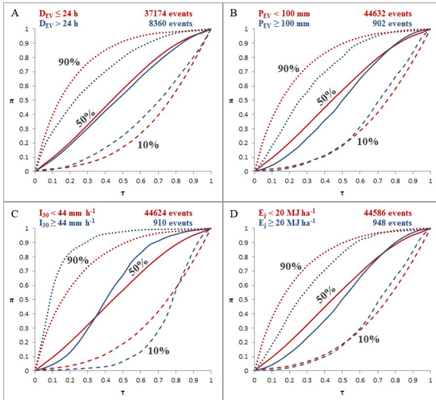
**Fig. 4.** Comparison between SRP of the 45 534 erosive events recorded in Calabria, distinguished by **(A)**  $D_{EV}$ , **(B)**  $P_{EV}$ , **(C)**  $I_{30}$ , and **(D)**  $E_J$ . The 90th, 50th, and 10th fractiles for each class are shown. On the horizontal axis,  $\tau$  represents the cumulative fraction of the rainstorm time; on the vertical axis,  $\pi$  represents the normalized cumulative depth of the rainstorm.
