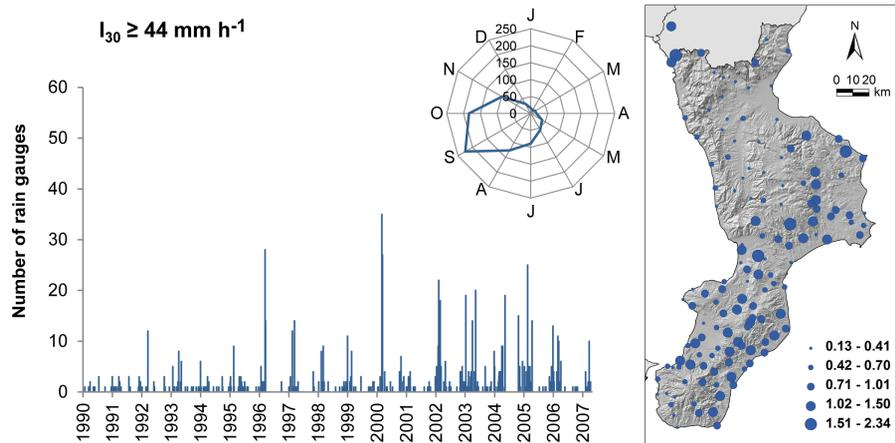
**Fig. 6.** Rainfall events characterized by  $I_{30} \geq 44 \text{ mm h}^{-1}$ : timeline of the number of rain gauges that exceed the threshold value. The numerosness of events for each month is shown in the inset. The location and the ratio between numerosness of rainstorms and number of observation months for each rain gauge is shown in the map on the right.
