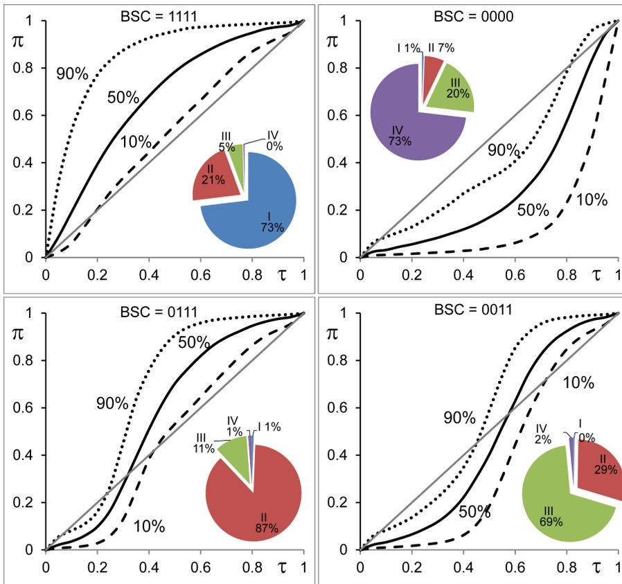
**Fig. 3.** Standardized Rainfall Profiles (SRP) relative to the 90th, 50th, and 10th fractiles of the four most numerous BSC in Calabria. In the insets, with reference to each BSC, Huff's quartiles are also distinguished. On the vertical axis,  $\pi$  represents the normalized cumulative depth of the rainstorm; on the horizontal axis,  $\tau$  represents the cumulative fraction of the rainstorm time.
