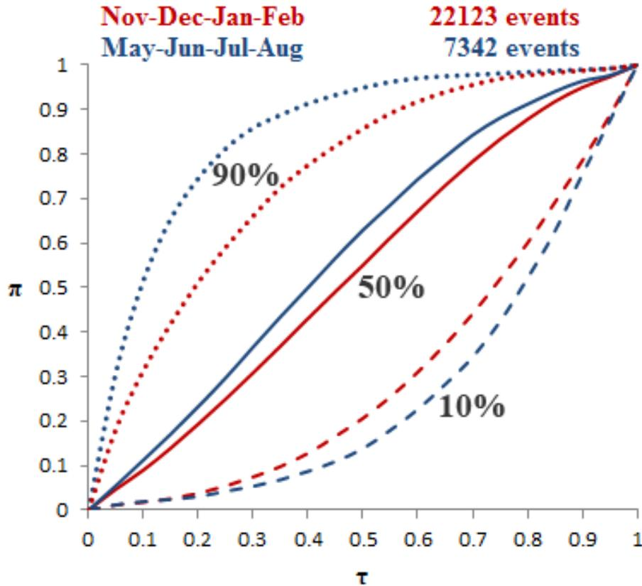
**Fig. 8.** Comparison between SRP of the events occurred during the four wettest and four driest months in Calabria. The 90th, 50th, and 10th fractiles for each class are shown. On the horizontal axis,  $\tau$  represents the cumulative fraction of the rainstorm time; on the vertical axis,  $\pi$  represents the normalized cumulative depth of the rainstorm.
