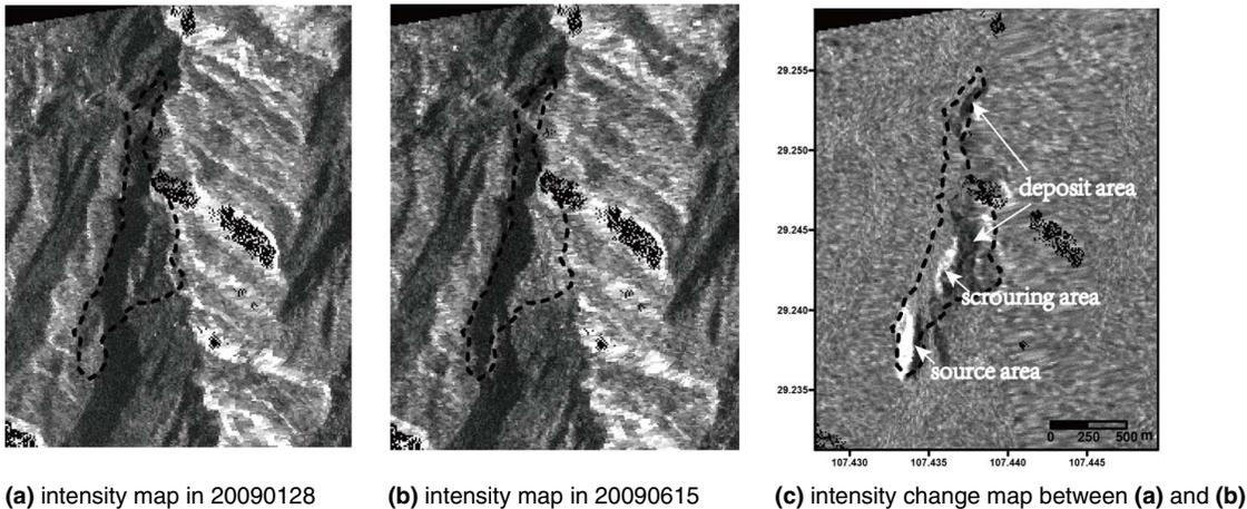
**Fig. 7.** Two SAR Intensity images acquired on 28 January 2009 (a) and 15 June 2009 (b). (c) Intensity change map between (a) and (b). Dashed polygon is superimposed on each map to indicate the affected area inferred from aerial photo. In (c), source area, scouring area and two deposit areas are indicated.
