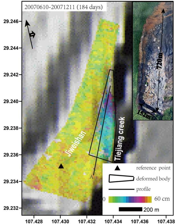
**Fig. 5.** The cumulative deformation map during 10 June and 11 December 2007 (184 days). The irregular polygon outlines the deformed rockslide body. Black triangle indicates the reference point for InSAR time-series analysis. Profile AB will be discussed in Fig. 6. The inset is the aerial photograph taken after Jiweishan sliding (Yin et al., 2011).
