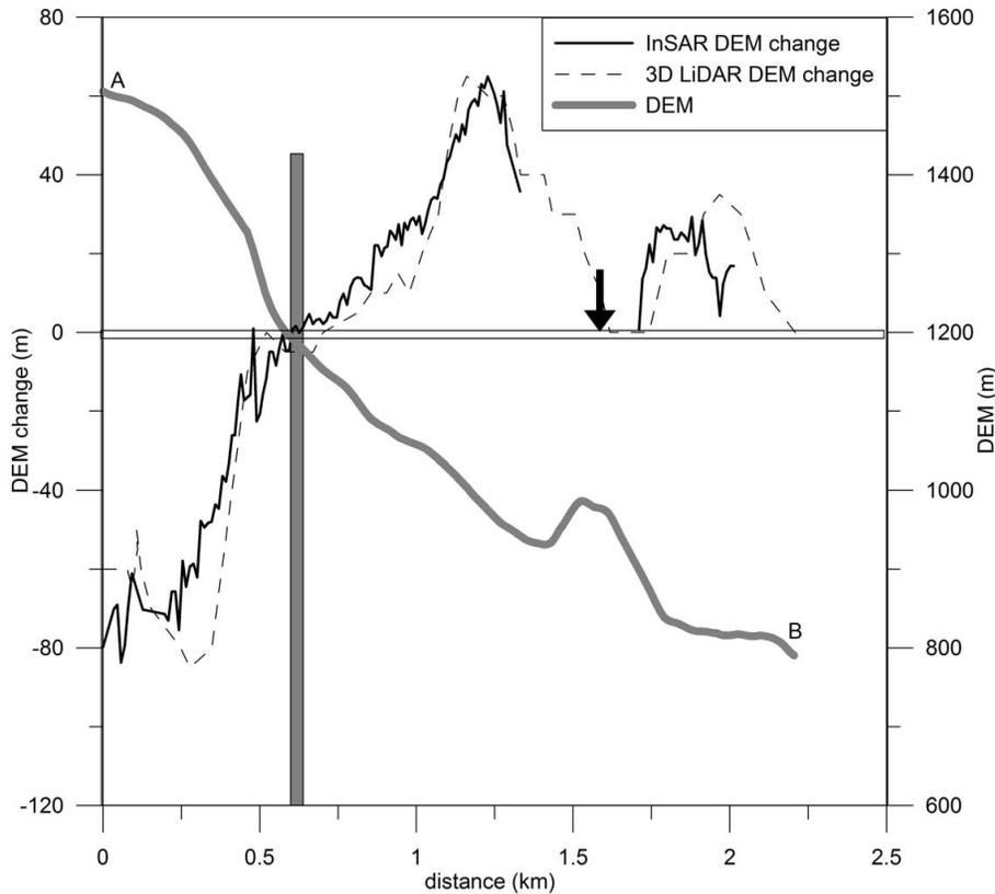
**Fig. 9.** Cross-section of pre-slide SRTM DEM, DEM change measured by InSAR and 3-D LiDAR techniques after Jiweishan sliding along profile AB. The vertical grey bar indicates the transaction point between the source area and the deposit area, while the black arrow shows the location of scouring region between two deposit areas.
