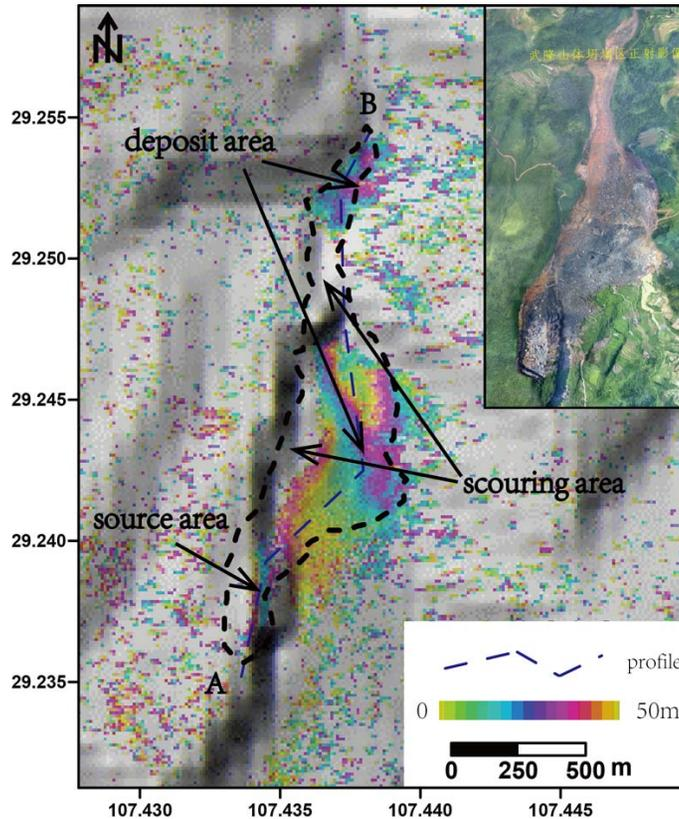
**Fig. 8.** DEM change map calculated by InSAR stacking method after Jiweishan sliding. The black dashed line delineates the affected region based on an aerial photo and the blue dashed line represents the location of the profile AB shown in Fig. 9.
