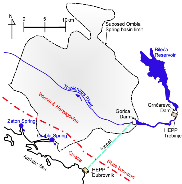
Fig. 1. Location map indicating the study area, the site of the Ombla Spring with its supposed catchment area, the Zaton Spring, the Trebišnjica River, the boundary limit between Croatia and Bosnia and Herzegovina, as well as the position of existent dams, reservoirs and HEPP-s.
