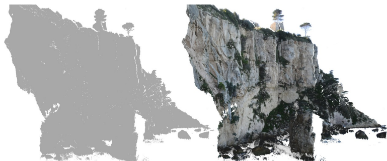
Fig. 5. TLS point cloud of the Mt. Pucci cliff: left: the standard point cloud; right: the point cloud colored by the optical photos.
