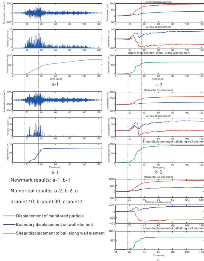
**Fig. 6.** Acceleration and displacement under shaking based on Newmark and numerical methods (the red and blue lines in the right column of Fig. 6 are the displacements of the monitored particles and boundary displacements, respectively. Positions of the disks shown in Fig. 4.).
