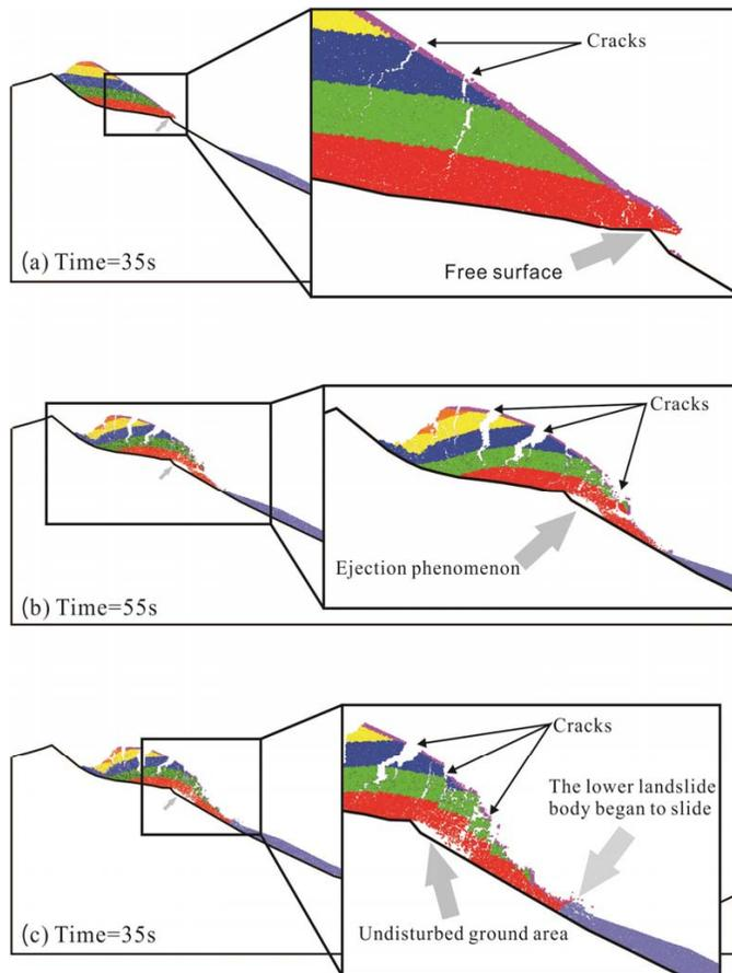
**Fig. 10.** Ejection phenomenon in the Donghekou landslide.
