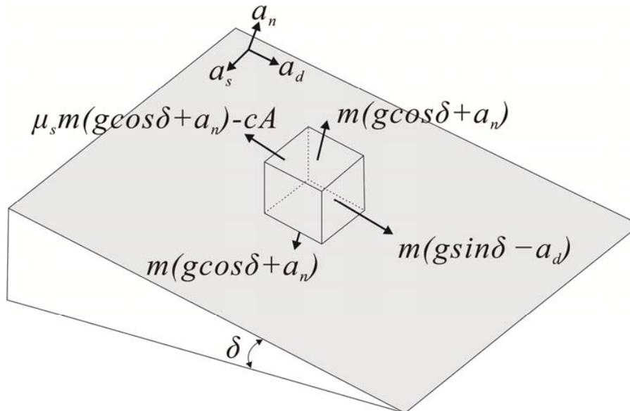
**Fig. 3.** Diagram illustrating the critical balance condition of forces exerted on a rock block lying on an inclined planar surface under the earthquake ground motion.
