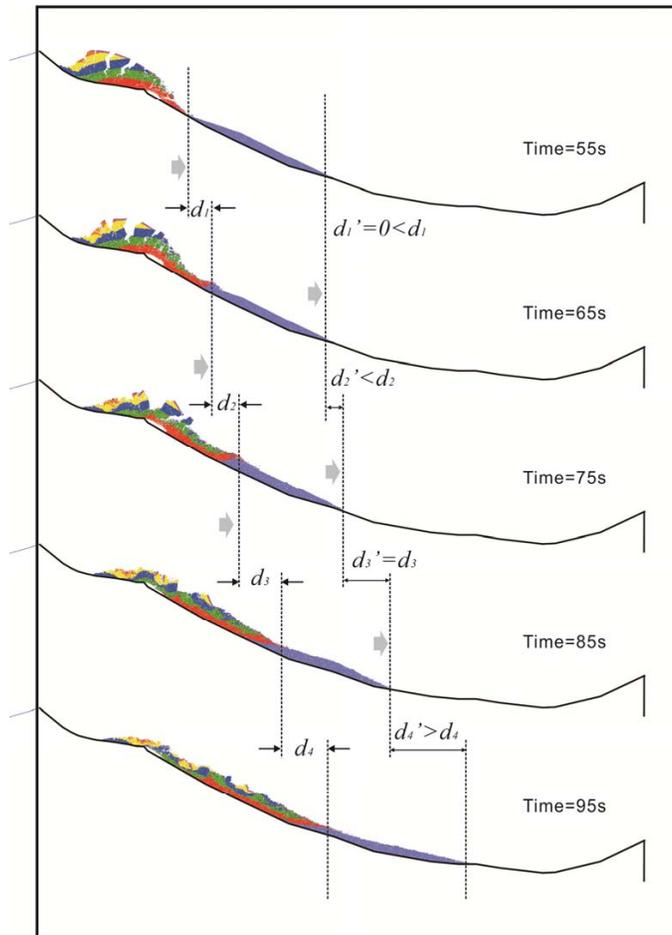
**Fig. 11.** Displacement changes in different parts of the lower landslide body.
