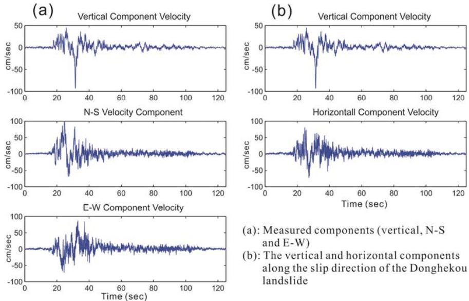
**Fig. 5.** Velocity diagram of the accelerometer station in Jiangyou during the Wenchuan earthquake.
