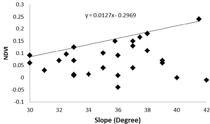
**Fig. 5.** Extraction of a relationship between the NDVI and the slope values for 26 debris flows within ephemeral streams that were verified in the field and/or by examination of Google Earth images. A linear regression was used to identify the equation of a straight line that best fitted the points with the steepest slope and the smallest NDVI values. Points plotting on or below the extracted line are susceptible to motion, whereas those above the line are stable.
