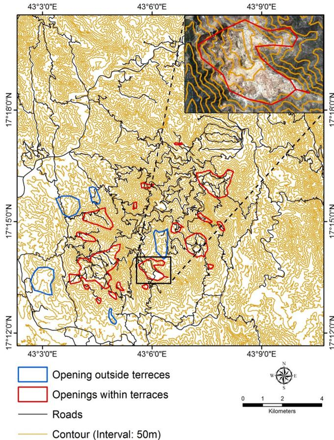
**Fig. 10.** Contoured elevation map showing locations of possible historical landslides; these areas appear as domains of gentle slope surrounded by areas with steep slopes.
