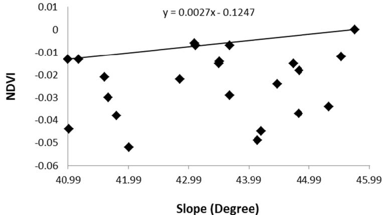
**Fig. 8.** Extraction of a relationship between the NDVI and the slope values for 21 overland debris flows on sparsely vegetated slopes that were verified in the field and/or by examination of Google Earth images. A linear regression was used to identify the equation of a straight line that best fitted the points with the steepest slope and the smallest NDVI values. Points plotting on or below the extracted line are susceptible to motion, whereas those plotting above the line are stable.
