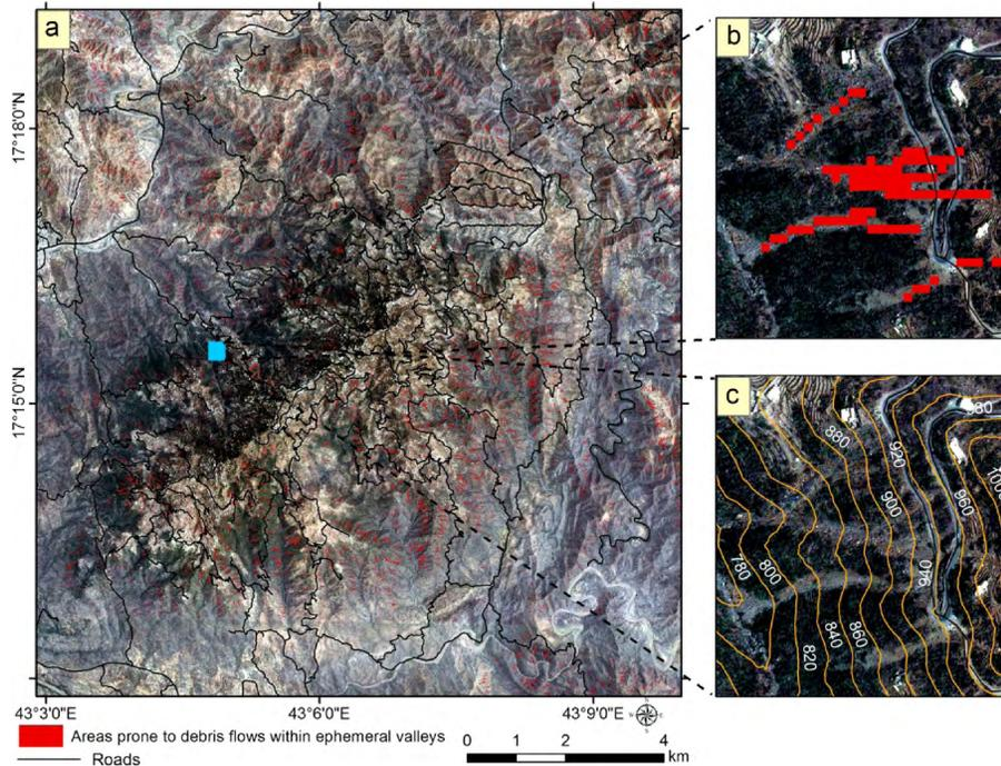
**Fig. 6.** (a) Hazard map showing the distribution of the areas modeled as being prone to debris flows within ephemeral streams (red areas). (b) Enlargement of the boxed area in (a). (c) Same as (b), but with the modeled debris flow omitted. Note the correspondence between the modeled (b; red areas) and observed (c: bright areas) debris flows.
