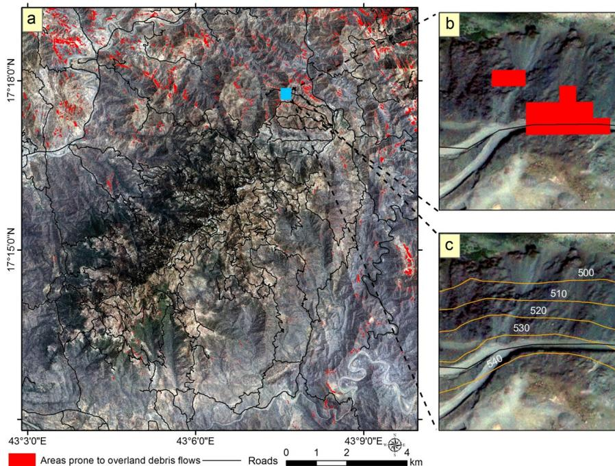
**Fig. 9.** Hazard map showing the distribution of areas prone to overland debris flows (red areas) related to the presence of sparsely vegetated steep slopes. **(b)** Enlargement of the boxed area in **(a)**. **(c)** Same as **(b)**, but with the modeled overland debris flows omitted. Note the correspondence between the modeled **(b):** red areas) and observed overland **(c):** bright areas) debris flows.
