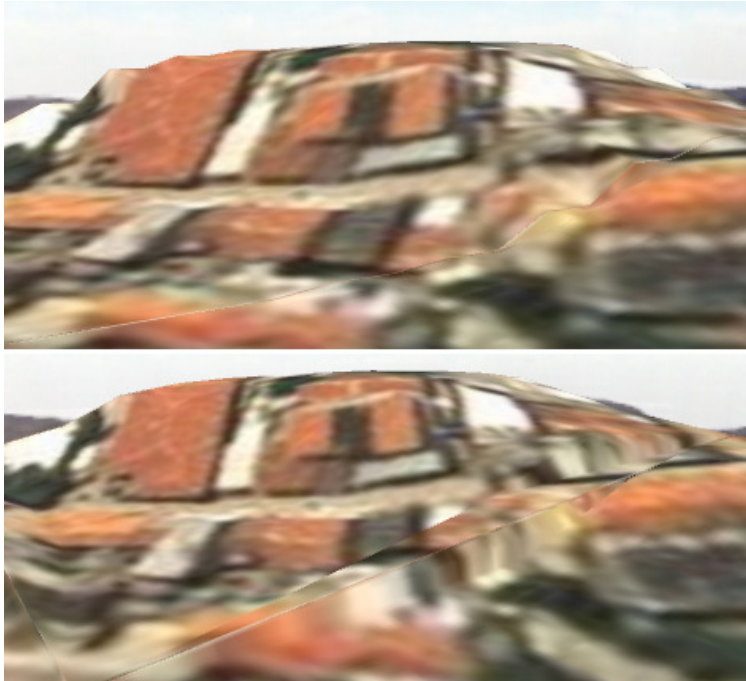
Fig. 16. Textured model with continuous smooth transitions (upper) and without continuous smooth transitions (bottom) between surfaces.
