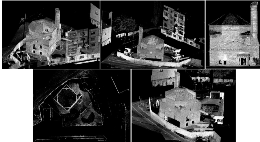
Fig. 4. Scan view of the structure from different scan stations.
