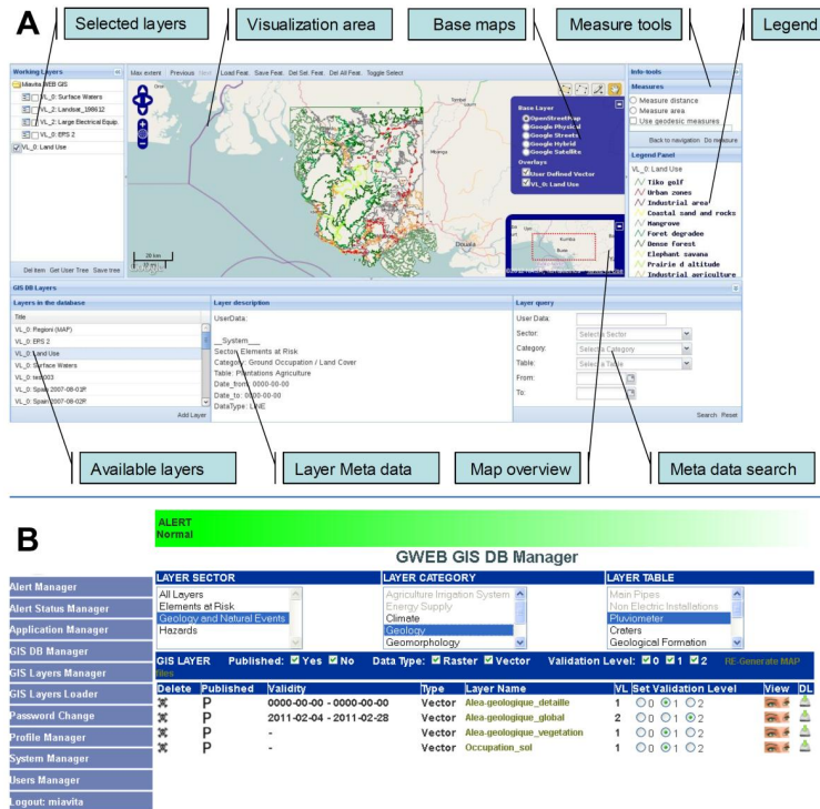
Fig. 8. (A) Represents the end user’s WEB interface completely programmed in Javascript and running on a standard WEB Browser. Different areas of the screen can be folded to give more space to the GIS central visualization area. The users can search the GIS database using the meta information stored along with the geographical data – screen bottom three panels. The selected GIS layers can be saved as independent scenarios and later retrieved from the server, as well as user’s vector features (polygons, lines and points) can be added to the visualization area, saved on the server for further use and shared with the other WebGIS users. (B) Shows the server GIS Layers Manager component. This module allows the management of all the GIS data contained in the database, including the promotion/demotion of the “validation level” associated with each GIS layer. In the left side the system shows all the management modules that allow the management and configuration of the whole system, including the switch from one Alert Level to another. Each Alert Levels can be independently configured giving GIS data access priority to the more appropriate users in case of emergency.
