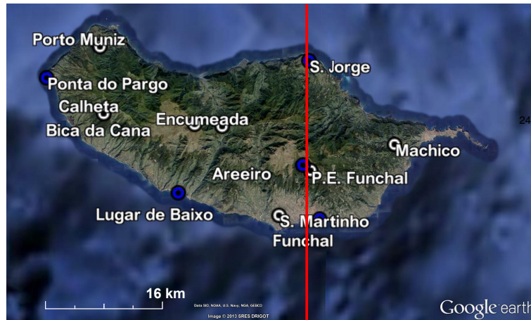
Fig. 3. Location of the weather stations in Madeira Island (blue dotted – Portuguese Meteorological Institute; White dotted – Madeira Regional Civil Engineer Laboratory) and the cross section at 16.93° W used in this work (red line).
