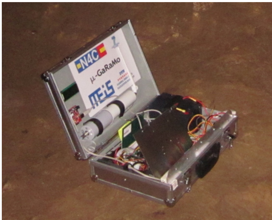
Fig. 7. Mobile DTN node based on Intel Atom embedded computer mounted in a simple case with radiological probe and simple LCD display presenting the current date and time, number of connections, number of bundles and last measured radioactivity (the node is measuring gamma dose rate for other purposes; its basic task in the experiment is to act as the mobile DTN “data mule” node for carrying data from cave to entrance).
