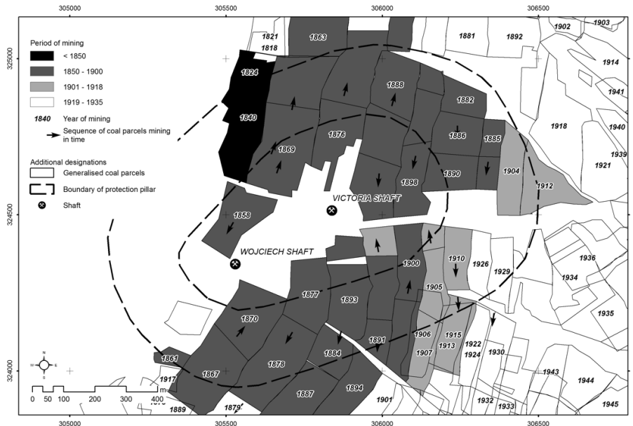
Fig. 10. Mining activity analysis for the 424/425 coal production level within the boundaries of the protection pillar.
