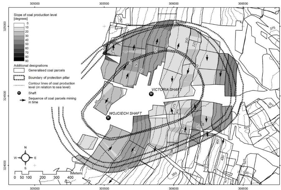
Fig. 11. Slope analysis for the 424/425 coal production level coal within the boundaries of the protection pilla.
