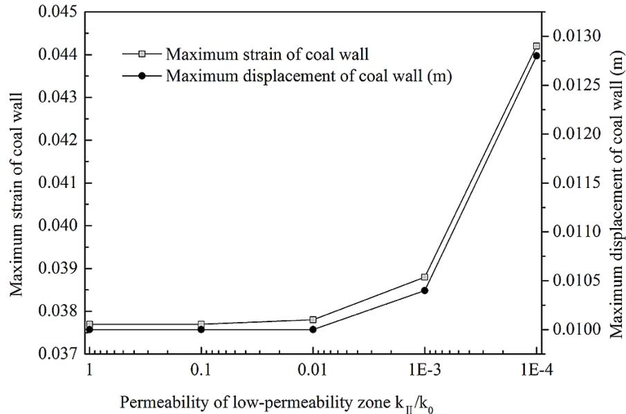
**Fig. 9.** Deformation of coal wall.
