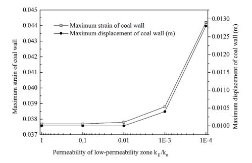
Fig. 9. Deformation of coal wall.
