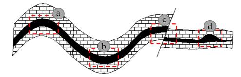
Fig. 1. Abundant zones of coal gas in some geologic structures.
