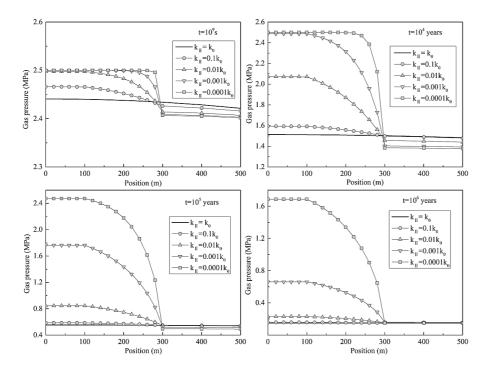
Fig. 4. Gas distributions with various permeability properties of the low-permeability zone.
