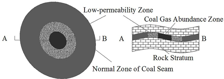
**Fig. 2.** Annular low-permeability zone in coal seam.
