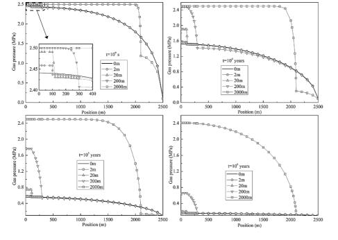
**Fig. 5.** Gas distributions with various lengths of the low-permeability zone.
