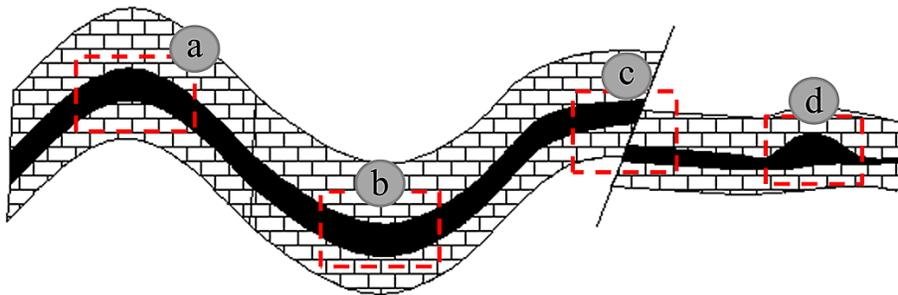
**Fig. 1.** Abundant zones of coal gas in some geologic structures.
