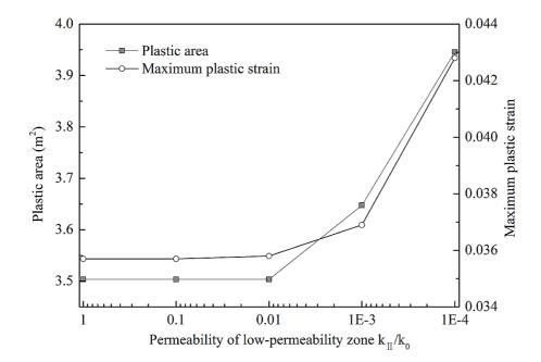
Fig. 8. Plastic development in front of coal wall.
