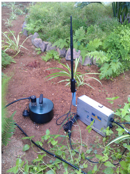
Fig. 12. Node deployed on the terrain with wireless antenna installed on the ground and geophone sensor.
