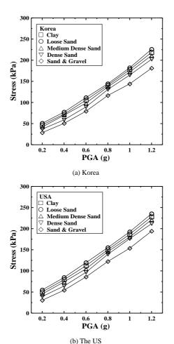
Fig. 8. Stress of brittle pipeline mobilized by earthquake loadings with respect to peak ground acceleration (PGA) in various in-situ ground conditions.
