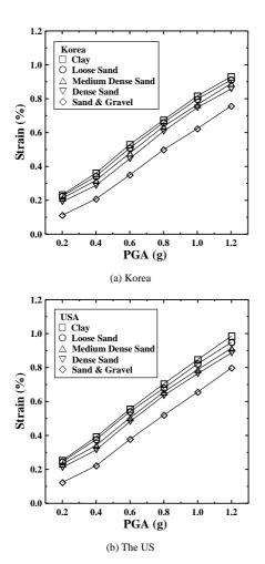
Fig. 9. Strain (%) of brittle pipeline mobilized by earthquake loadings with respect to peak ground acceleration (PGA) in various in-situ ground conditions.
