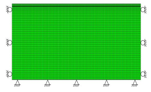
Fig. 5. Finite element mesh configuration and boundary conditions for pipelines.
