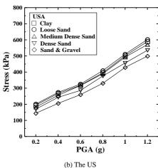
**Fig. 6.** Stress of ductile pipeline mobilized by earthquake loadings with respect to peak ground acceleration (PGA) in various in-situ ground conditions.
