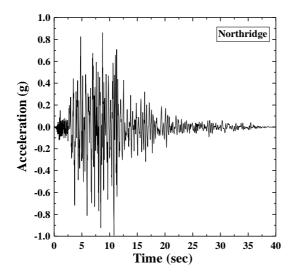
Fig. 2. History of ground acceleration record during Northridge earthquake (COSMOS, 2010).
