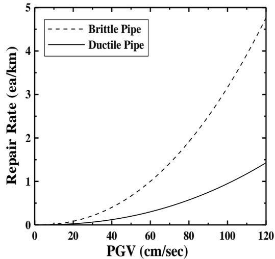
**Fig. 1.** Fragility curve of buried pipelines provided by HAZUS (FEMA, 1999).
