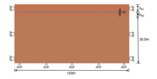
Fig. 4. Configuration of numerical model associated with pipeline and ground conditions.
