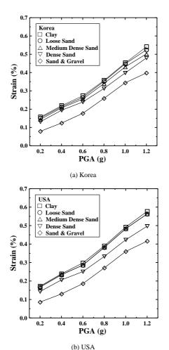
Fig. 7. Strain (%) of ductile pipeline mobilized by earthquake loadings with respect to peak ground acceleration (PGA) in various in-situ ground conditions.
