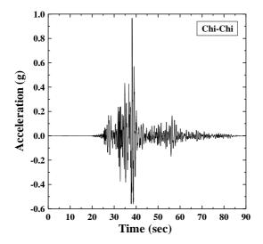
Fig. 3. History of ground acceleration record during Chi-Chi earthquake (COSMOS, 2010).
