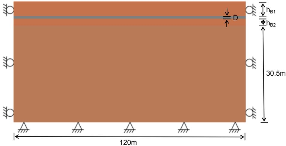
Fig. 4. Configuration of numerical model associated with pipeline and ground conditions.
