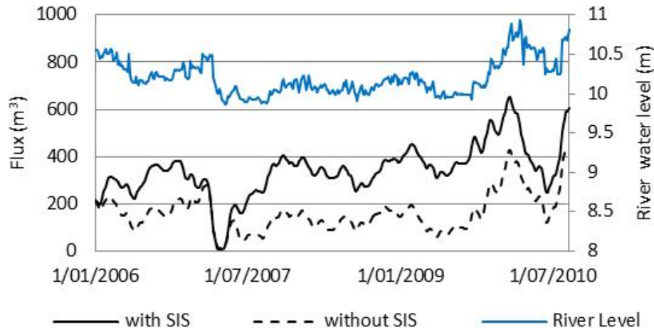
Fig. 9. Results of water flux from the river to the floodplain aquifer for the defined scenarios.
