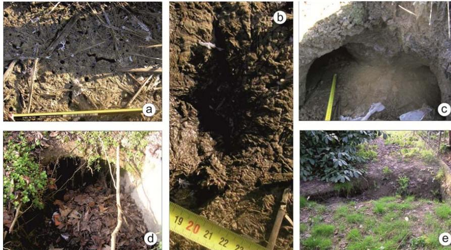
**Fig. 10.** Supposed evolution steps in micro-sinkholes formation: **(a)** little holes of water circulation along soil fractures; **(b)** partial hollow zone; **(c)** vault fall showing horizontal tunnels; **(d)** horizontal tunnels; **(e)**: gully.
