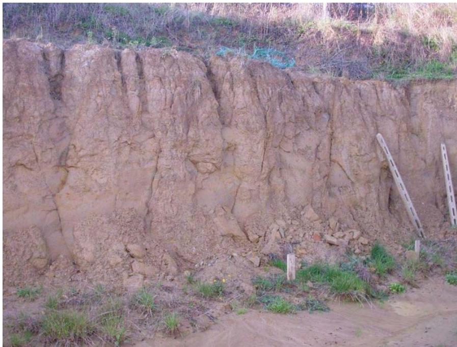
**Fig. 5.** An example of deep soil cracks affecting clay deposit near Paganico (the scarp is approximately 2 m high).
