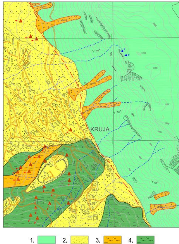
Fig. 15. Slope stability zonation map of Kruja town in case of arid period, scale 1 : 5000. (1) engineering geology zone with basement of limestones rocks, stable, (2) engineering geology zone with basement of breccia's rocks, stable, (3) engineering geology site in critical state, (4) engineering geology site in stable state.
