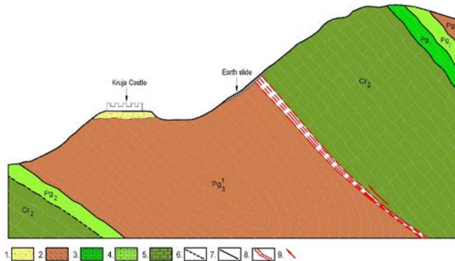
Fig. 2. Geological profile of Kruja region (Xhomo et al., 2002; Muceku, 2008). (1) breccia's rocks, (2) flysch rocks, (3) limestone rocks of Paleocene (Pg 1 ), (4) limestone rocks of Eocene (Pg 2 ), (5) limestone rocks of Upper Cretaceous (Cr 2 ), (6) stratigraphic break's boundary, (7) normal boundary, (8) overthrust tectonics, (9) mass movement direction.
