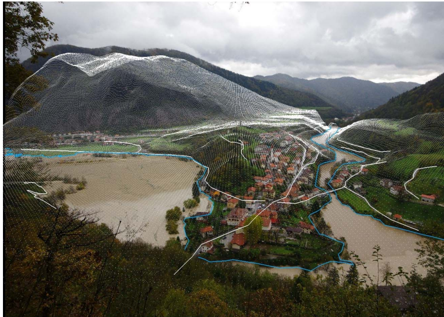
Fig. 2. Digital terrain model (white), roads (white) and border of the flooded area (blue) superimposed on the image of the floods in Most na Soči on 5 November 2012 around 13:00 (marked with (b) on Fig. 1). The author of the underlying image is Miljko Lesjak.
