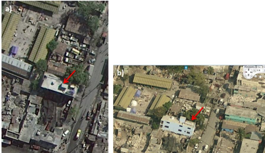
**Fig. 2.** Example of a building suffering from a soft storey failure observed on the aerial imagery **(a)** and on the oblique Pictometry image **(b)**. The lateral view provided by Pictometry data allows a better detection of this type of damage.
