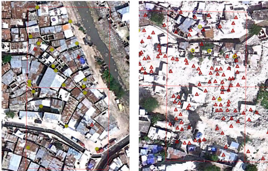
**Fig. 7.** Examples of (left) overestimation of MTPTC surveyed points (yellow circles) versus UWJ damage points (red triangles) for the highly damaged and destroyed categories and (right) underestimation. The background image is © Google Earth, 2010.
