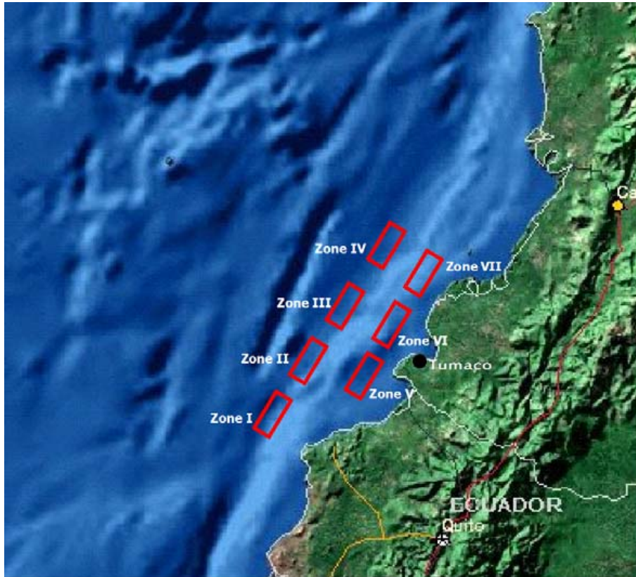
Fig. 5. Potential sources (epicentres) of tsunami generation for the southern Colombian Pacific coast defined from studies developed by Beck and Ruff (1984), Mendoza and Dewey (1984), Gutsher et al. (1999), and Collot et al. (2004).
