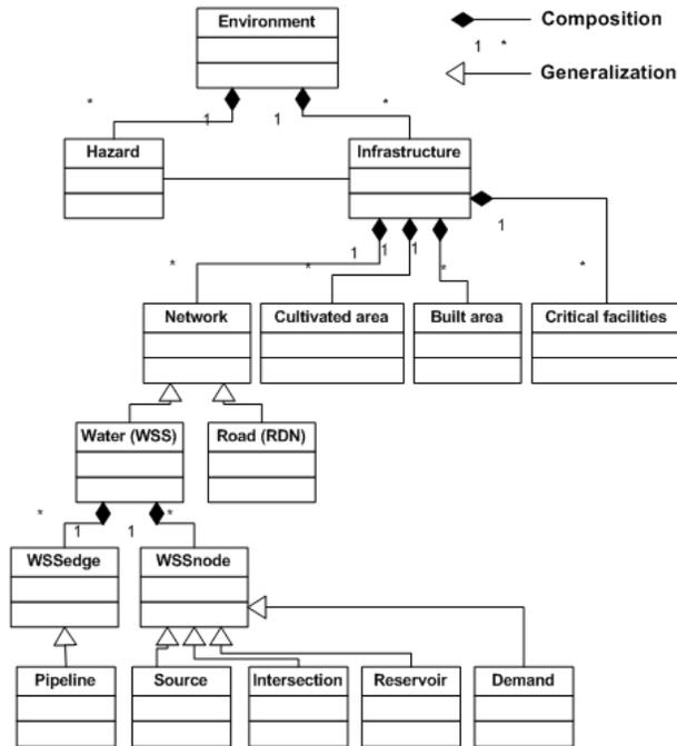
**Fig. 2.** UML class diagram of the studied infrastructure, adapted from Cavalieri et al. (2012).
