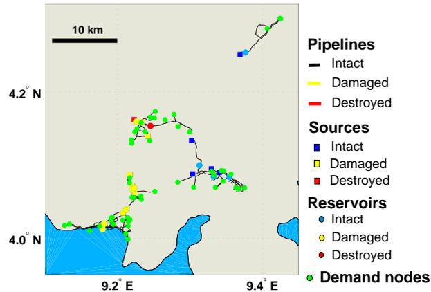
**Fig. 11.** Representation of the damage states of the water supply system components after the scenario presented in Fig. 5.
