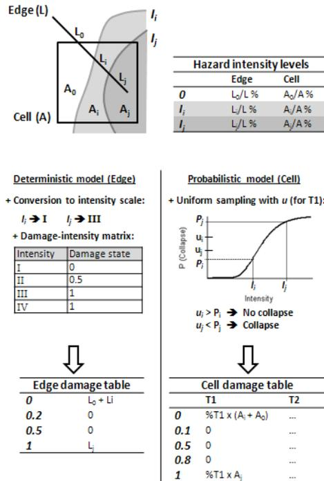
**Fig. 4.** (Top) Hazard projection procedure on linear and area-like vulnerable sites and (Bottom) Example of damage analysis for a hypothetical case, where the edge is assigned a deterministic model, and the cell contains a proportion %T1 of building typology 1, with a collapse fragility function.
