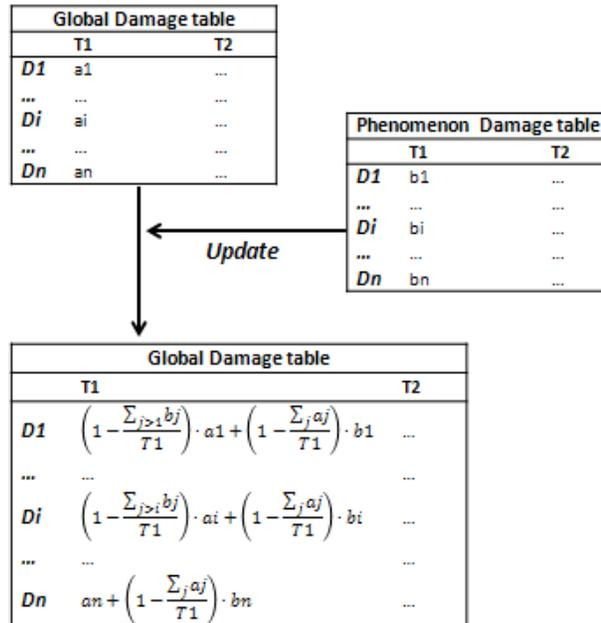
**Fig. 6.** Update procedure for a cell object (the same applies for edges), containing the building typology 1 over an area  $T_1$ .  $a_i$  and  $b_i$  represent the areas of impacted buildings.  $D_i$  is the damage state, according to an hypothetical damage scale.
