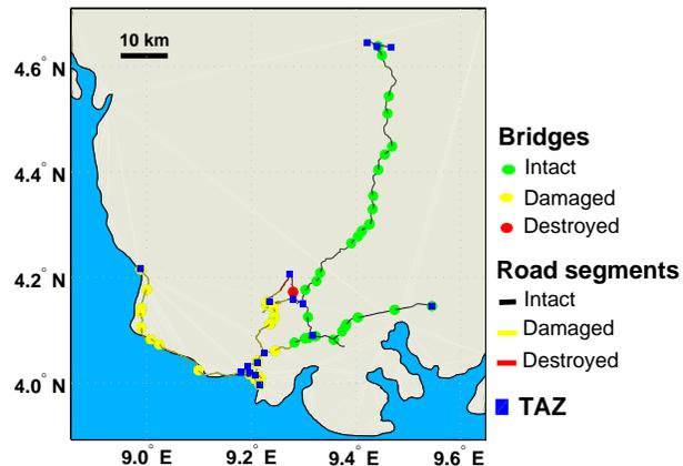
**Fig. 10.** Representation of the damage states of the road network components after the scenario presented in Fig. 5.
