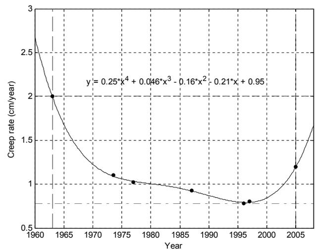
**Fig. 4.** Creep rates determined at Ismetpasa and their prediction. Creepmeter resolution in 1986 is not used for the prediction because it seems to be outlier in the creep history.
