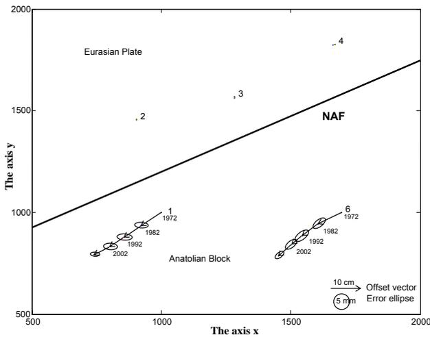
**Fig. 3.** Surface displacements at points 1 and 6 relative to Eurasian plate since 1972. The axes are plotted on the Gauss-Krüger projection plane. The arrows and ellipses are the offsets and the error ellipses of the offsets, respectively. Their scales are shown at the right lower corner. The solid line is the NAF.
