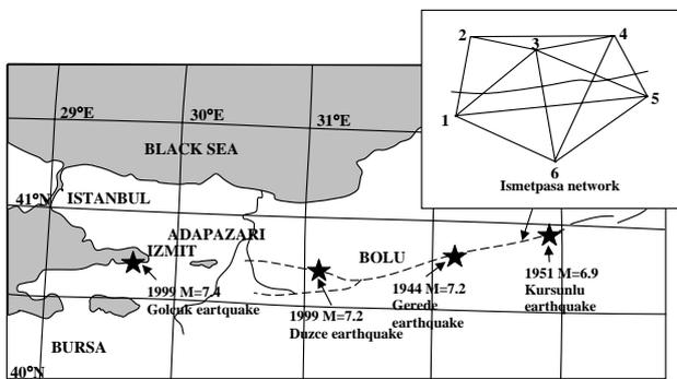
**Fig. 2.** Map of the NAF around the Marmara and the Northern Black Sea region (adapted from Deniz et al., 1993). The inset map shows the Ismetpasa geodetic network. As for the scale of the inset map, the distance between the points 1 and 5 represents 1.2 km in field. The dashed line is the trace of the NAF. The stars locate the major earthquakes that occurred in the last century.
