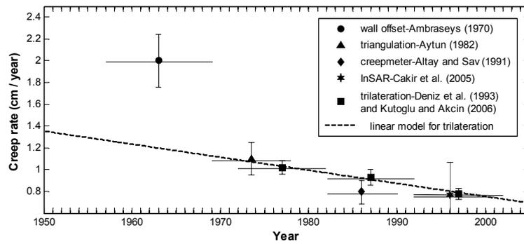
**Fig. 1.** Creep rates for the Ismetpasa segment obtained from different studies (adapted from Cakir et al., 2005). Horizontal bars represent the time window. Vertical bars shows the error ranges.
