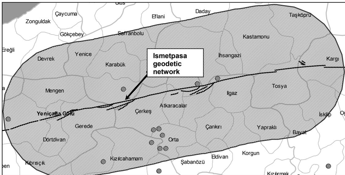
**Fig. 5.** Earthquakes with the magnitude of 4 and over occurred in the 50 km near zone of the Ismetpasa segment after 2002. The dashed area shows the 50 km zone. The solid circles are the earthquakes (adapted from Sayisal Grafik, 2008).
