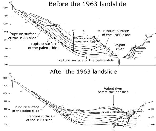
**Fig. 8.** Sections of the Vajont valley before and after 9 October 1963, landslide. The presence of paleo-slide at the Toc mountain is visible in both the panels, presenting a rupture surface very close to the rupture surface of the 1963 slide. A section of the landslide occurred in 1960 is also visible in the left panel (picture taken from Semenza, 2002).
