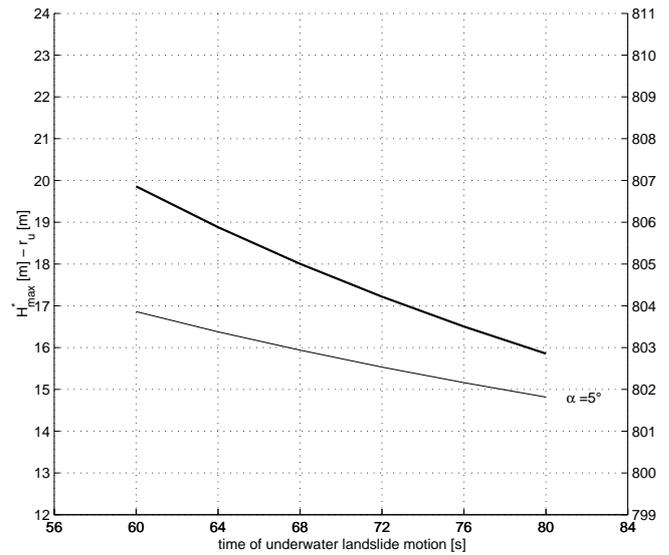
**Fig. 6.** Estimated maximum wave height  $H_{\max}$  and runup  $r_u$  generated by the landslide event of 22 March 1959, at the Pontesei reservoir. The secondary y-axis refers to levels above the m.s.l.
