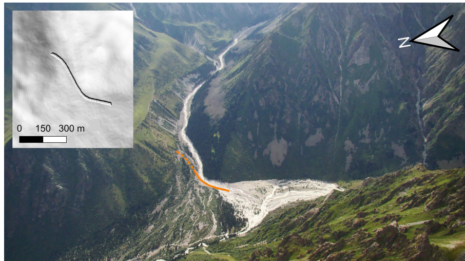
Figure 4. Photograph of the Aksay fan with the position of the existing deflection dam as of 2024 (solid orange line) and the enhanced deflection dam (dashed orange line). Top left box: Hillshade of the artificially modified DEM produced for the RAMMS simulation of the DRM measure. Bottom box: Profile across the river bed and the artificially enhanced deflection dam. Photograph: Vitalii Zaginaev, 2015.
