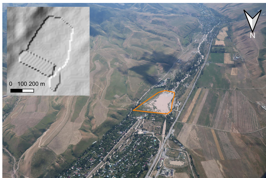
Figure 5. Photograph of the dam and retention basin (outlined in orange) in the village of Kashka Suu. Box top left: Hillshade of the artificially modified DEM for the RAMMS simulation of the DRM measure of the retention basin. Photograph: Vitalii Zaginaev, July 2024.
