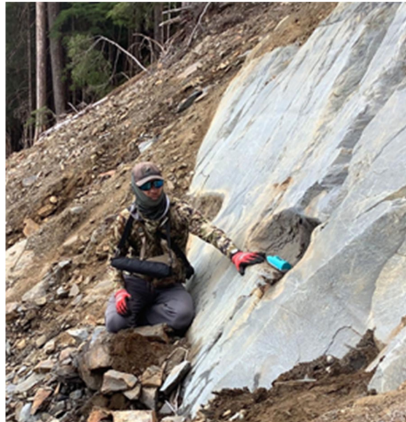
Figure S1. Image of Schmidt hammer readings being collected at the head of the MP11.2 landslide.
