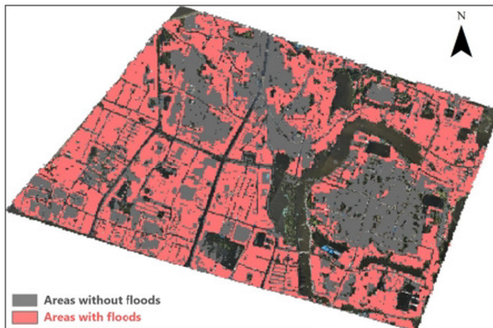
Figure 7. Flood monitoring results in the building area of Weihui City based on Sentinel-1 images and the Z-score method (Sentinel-1 data courtesy of ESA Copernicus). Grey indicates that the area has not been affected by the flood; red indicates that the area has been affected by the flood. The UAV imaging range is shown in Fig. 1.
