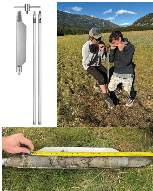
Figure 4. Russian Peat Auger (RPA) used in the field. The auger is pushed into substrate (top-right), and rotated to close the gate, isolating the sediment core from the substrate.
