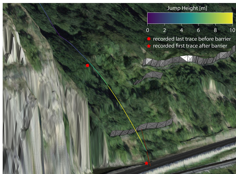
Figure A2. Three-dimensional simulation of a representative sliding deadwood trajectory at the Rothenbrunnen site. The figure shows the simulated log position at the time step when the log first touches the terrain after the jump over the barrier. The jump is initiated by a local plateau upslope of the barrier, leading to a maximum jump height of 9.9 m (measured as the vertical distance between the log centre of mass and the terrain) and a velocity of 27.8 \text{ m s}^{-1} at take-off. Background orthophoto from swisstopo (2020–2024).
