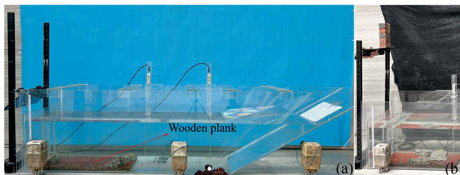
Figure 3. Photographs of the setup, (a) Experimental flume, (b) platform for inducing rotational cliff collapse.
