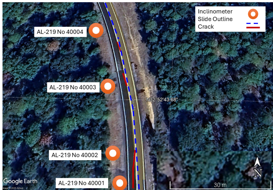
Figure 4. Location of four inclinometers at the AL-219 site in Centerville, Alabama, and cracks caused by the landslide (base map: Image © 2025 Airbus; Google Earth).
