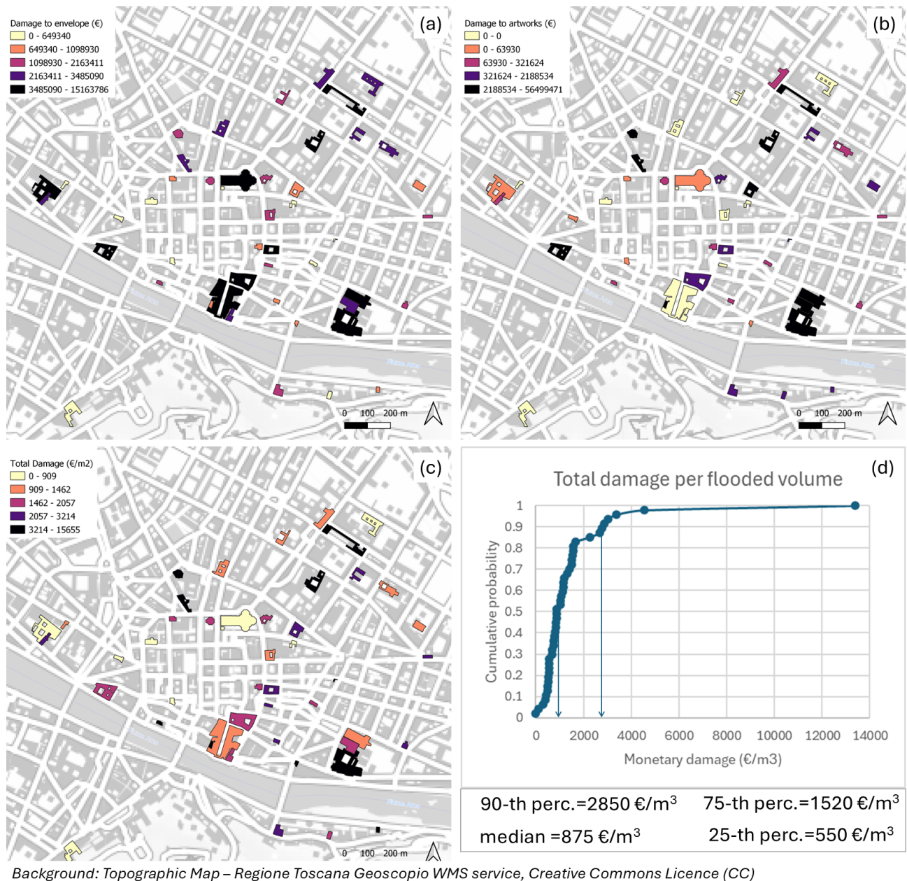
Figure 8. Monetary damage to CH envelope (a), artworks (b), unitary surface damage (c) and unitary volume damage (d). Background maps are based on data from OpenStreetMap. © OpenStreetMap contributors, licensed under the Open Database License (ODbL).
