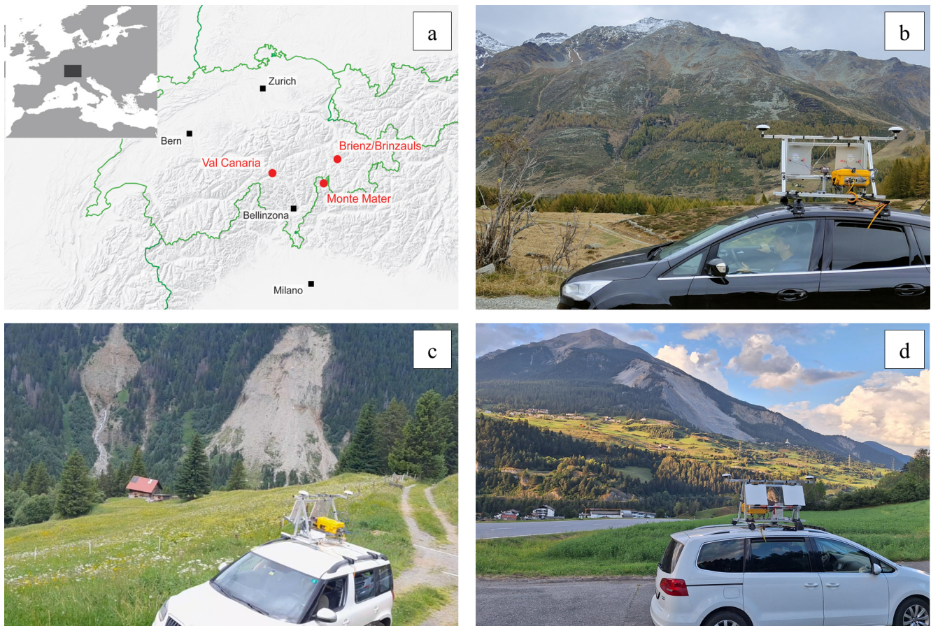
Figure 1. (a) Spatial context of the three selected study sites in the European Alps. Val Canaria (Canton Ticino) and Brienz/Brinzauls (Canton Grison) are located in Switzerland, Monte Mater (Lombardia) is located in northern Italy. (b) The Monte Mater rock slope instability in Italy with the GAMMA L-band SAR (GLSAR) instrument mounted on a car in the foreground. (c) The Rütan dei Sass landslide in Val Canaria with the car-borne GLSAR instrument in the foreground (cf. Sect. 3.2). Note that the measuring antennas do not face towards the landslide for illustration purposes only. (d) The Brienz/Brinzauls landslide complex with the car-borne GLSAR instrument in the foreground. Note that the measuring antennas face towards the viewer for illustration purposes only.
