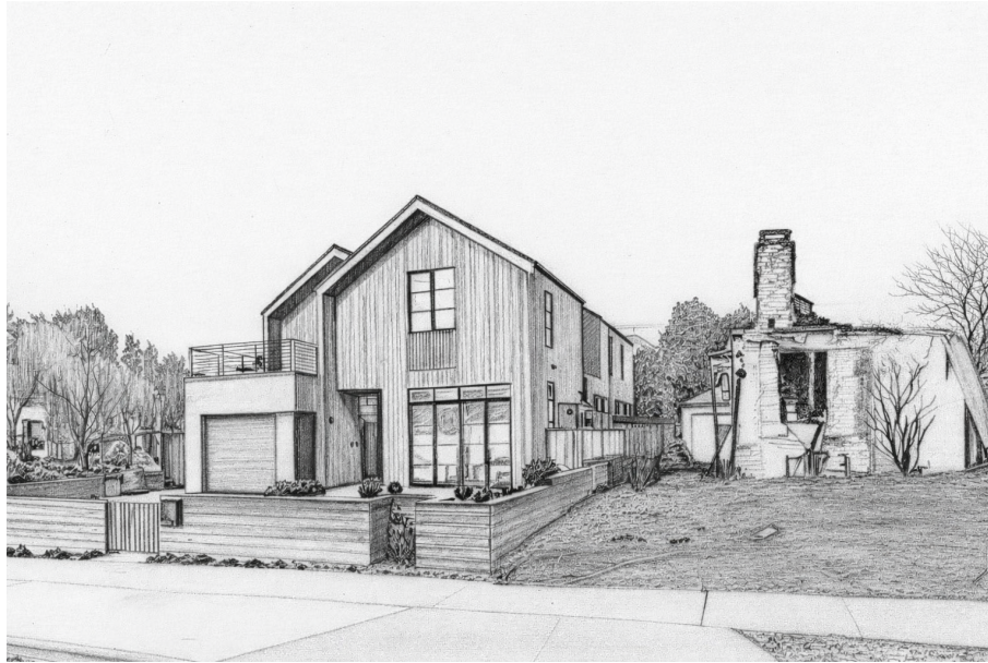
Figure 1. The sketch shows a wildfire-surviving house in Pacific Palisades, Los Angeles, constructed according to wildfire-resistant design principles. It is illustrating the concept of a non-combustible or fire-resistant exterior façade, helping to reduce ignition from radiant heat and wind-driven embers. Multi-pane windows are used to increase resistance to heat exposure and minimize breakage. The design includes adapted roof overhangs, sealed eaves, and ember-resistant detailing that limit pathways for embers to enter the structure. Gutters are designed to reduce debris accumulation, further lowering fire risk. Further details for reducing vulnerability are described in Papathoma-Köhle et al. (2022, 2025). Together, these architectural strategies contributed to the building’s remarkable performance during the 2025 wildfire events. Figure conceptualized from a Google Street View scene (February 2025).
