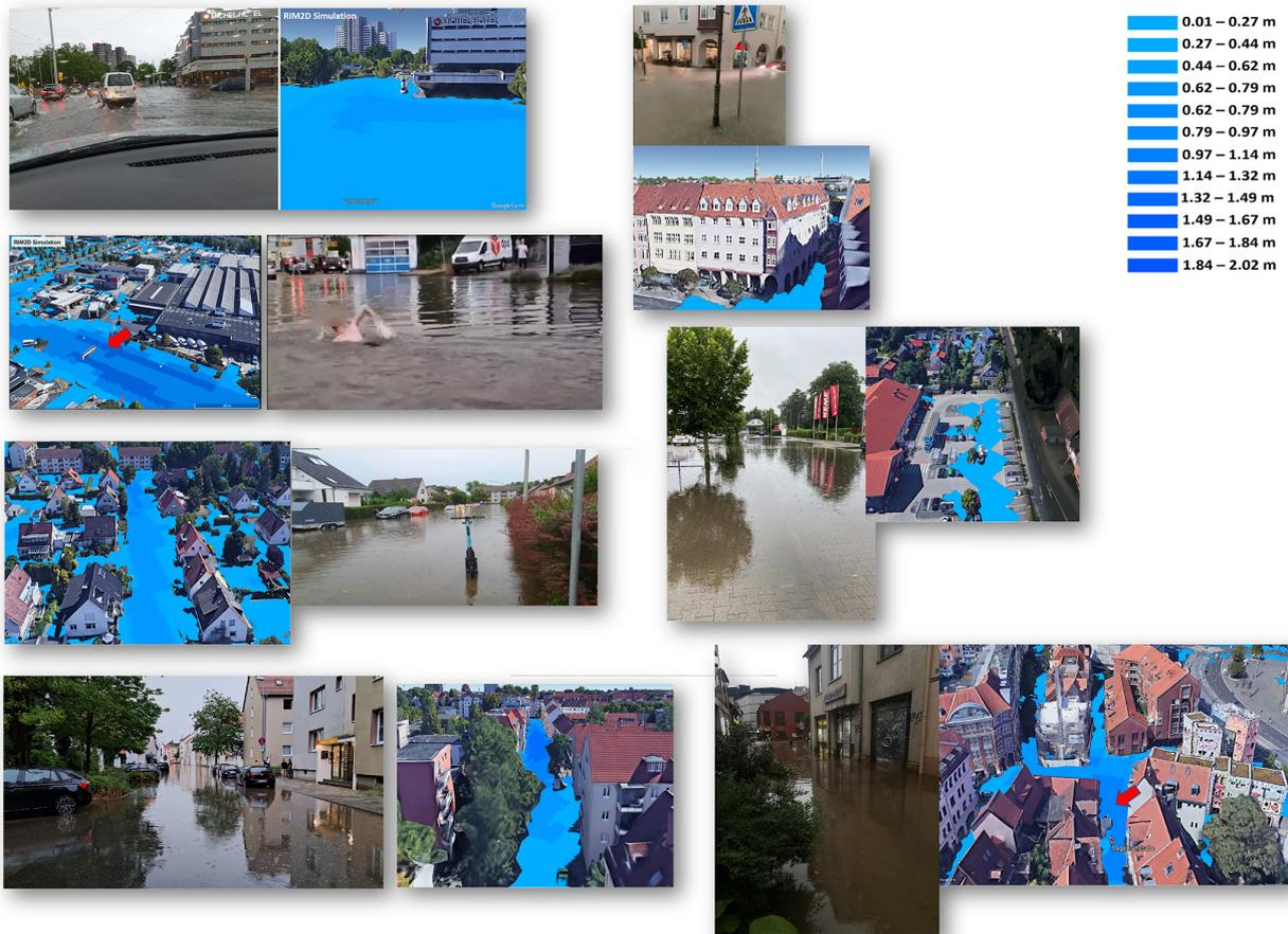
**Figure B1.** Examples of comparisons between the  $dx = 5$  m RIM2D simulation results and social media posts. Visualization of the RIM2D results and the background imagery are performed with and provided by Google Earth. Satellite imagery: © Google Earth 2024.
