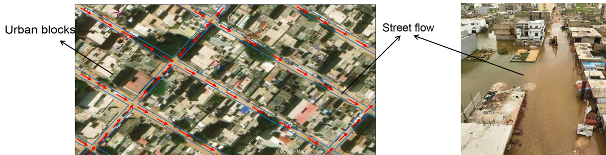
Figure 7. Surface water drainage paths at the urban street level. Background images © Google Maps 2023.
