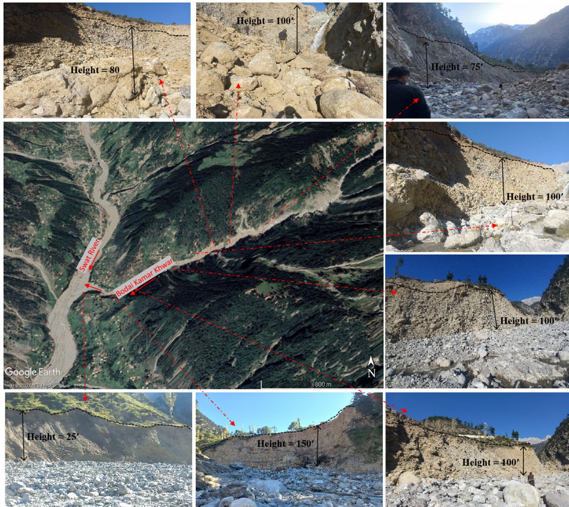
Figure 6. Through field investigation, identified source areas, stream erosion, and landslide deposits contributing to debris flow events at Bodai Kamar (DF 2) locations throughout the event. The background image for Bodai Kamar Khwar is taken from © Google Earth and for the other panels during the field visit.
