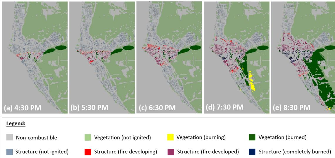
**Figure 2.** (a–e) SWUIFT simulation results at regular time intervals showing fire spread inside Lahaina, HI, on 8 August 2023. The colors indicate non-combustible areas (e.g., roadways), the status of vegetation (not ignited, burning, burned), and structures (not ignited, fire developing, fire developed, completely burned).
