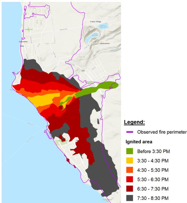
**Figure 3.** Fire perimeters from the SWUIFT simulation at 1 h intervals compared against the observed final fire perimeter.
