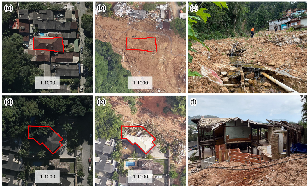
Figure 2. Examples of total destruction and partial damage to buildings. (a) Pre-disaster aerial view of a building that was totally destroyed. (b) Post-disaster aerial view of the total destruction to the building in (a). (c) Photograph from a field visit at the site where the building in (a) was located, taken in November 2023. (d) Pre-disaster aerial view of a building that was partially damaged. (e) Post-disaster aerial view of the partial damage to the building in (d). (f) Photograph from a field visit of the remnants of the building in (d), taken in November 2023. Data source: aerial imagery from DataGEO (2023).
